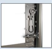
Cable break safety device. When the cable is broken or when there is an attempt to lift the doors without authorization, the device engages the strip, mounted on the door leg. At the same time the leaf is blocked. Consequently, the doors fall or their unauthorized lift is prevented.
