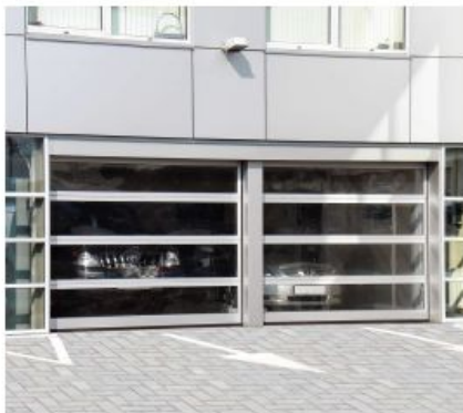
Glazed panoramic panels of aluminum sections form a door leaf.
